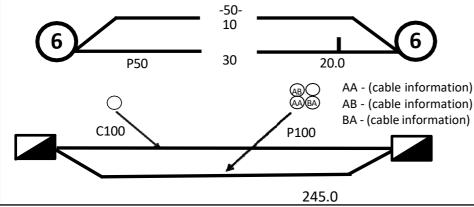
One 50mm PVC conduit (P50) containing a 50-pair and a 10-pair cable between two 6-pits. approximately 20.0m apart, with a direct buried 30-pair cable along the same route
